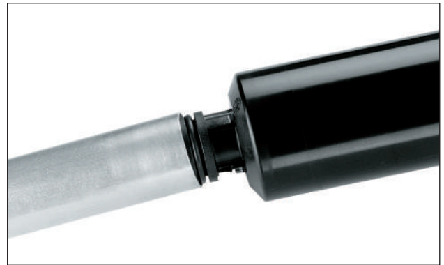
2. Attach the aluminum pipe to the outlet port and push it down to the stop.
