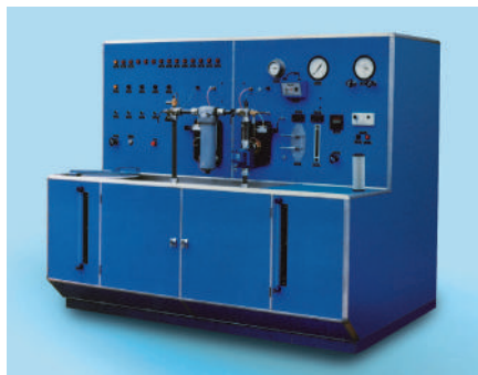
Multi-Pass test rig
