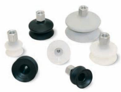
The cups described in this page, unlike the previous ones, are vulcanised onto an aluminium hexagonal support with a male or female threaded connector, inside of which there is an M8 threaded hole for the possible insertion of a calibrated grub screw (see page 1.118).
