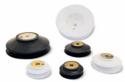
The main feature of these BELLOW CUPS is that they quickly crumple up during the grip, thus lifting the load for a few centimetres, independently of the movements of the lifting frame; this quick movement avoids that the load beneath, remains stuck to the lifted one.
